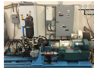
Hydraulic Hybrid Transmission HIL Test Rig with Electric Engine and Vehicle Emulators
